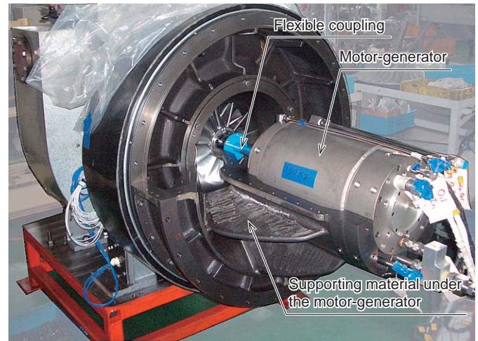
Fig. 5 Hybrid Turbocharger under assembling
